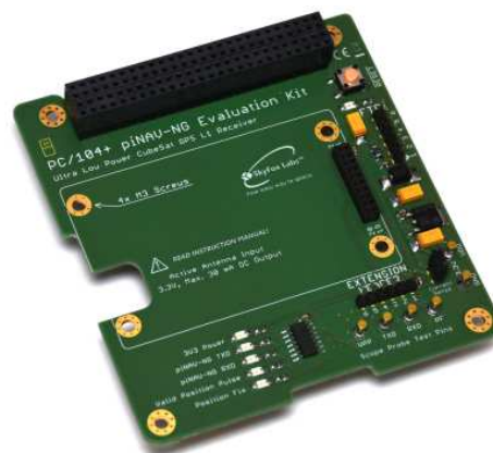
Fig. 10 The piNAV-NG PC/104+ Form Factor Evaluation Kit PCB Unit for development purposes (not for flight).
