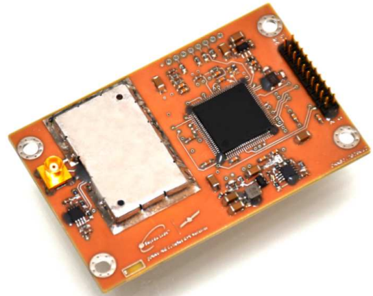
Fig. 1 CubeSat GPS Receiver - Next Generation (piNAV-NG), Flight Model, Top side view.
